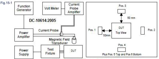
Figure 19: Magnetic Immunity Test Setup
