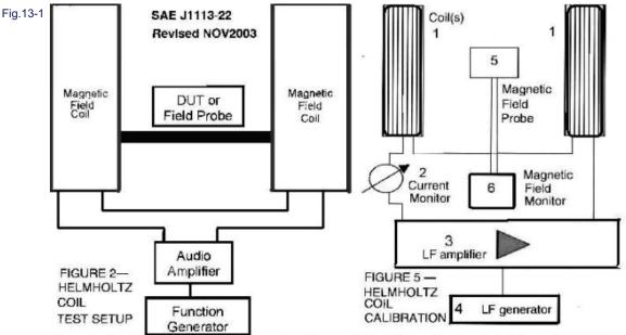
The current carrying capability and number of turns of the coil should be selected such that the test specification can be met. The coil should not have a self resonant frequency at or lower than the upper harmonic frequency of 30 kHz.
