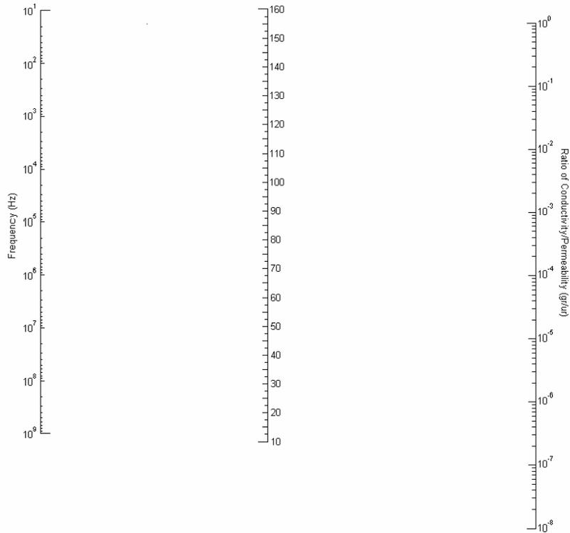
Figure 2c. Reflection Loss Nomograph for Plane Wave
