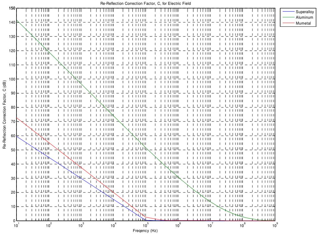
Figure 15. Re-Reflection Correction Factor for Electric Field
