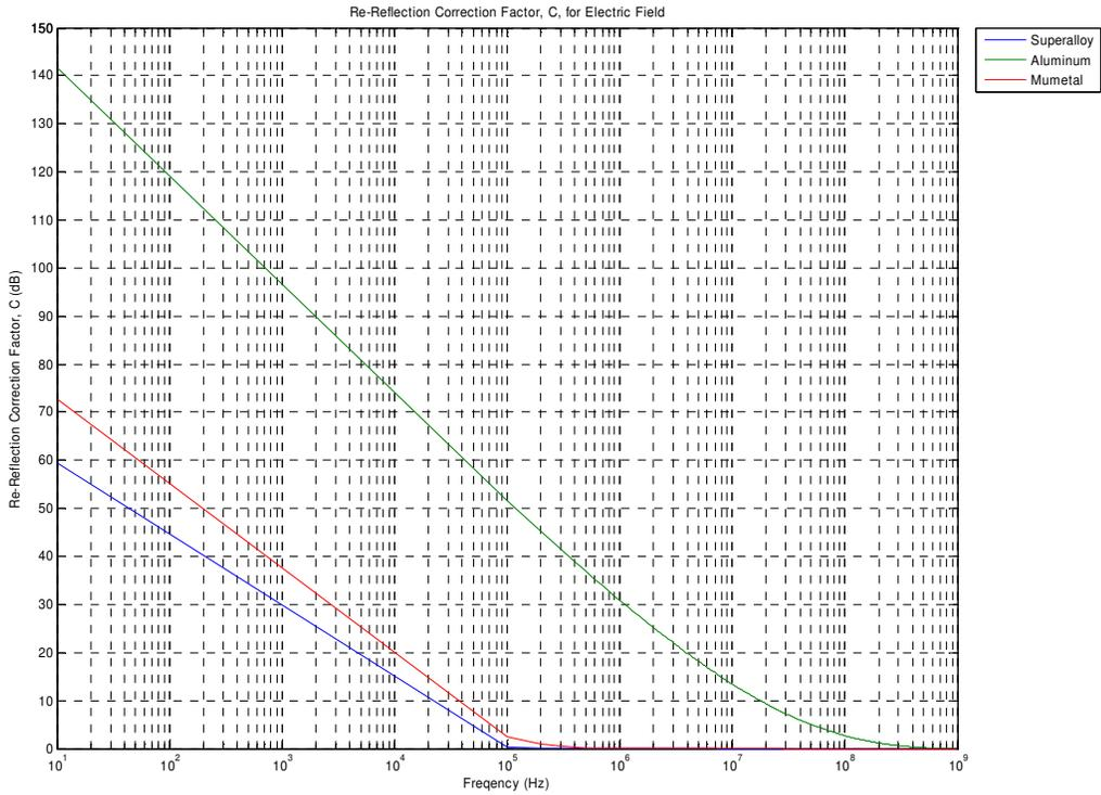
Figure 16. Re-Reflection Correction Factor for Plane Wave
