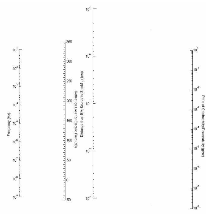
Figure 2b. Reflection Loss Nomograph for Electric Field
