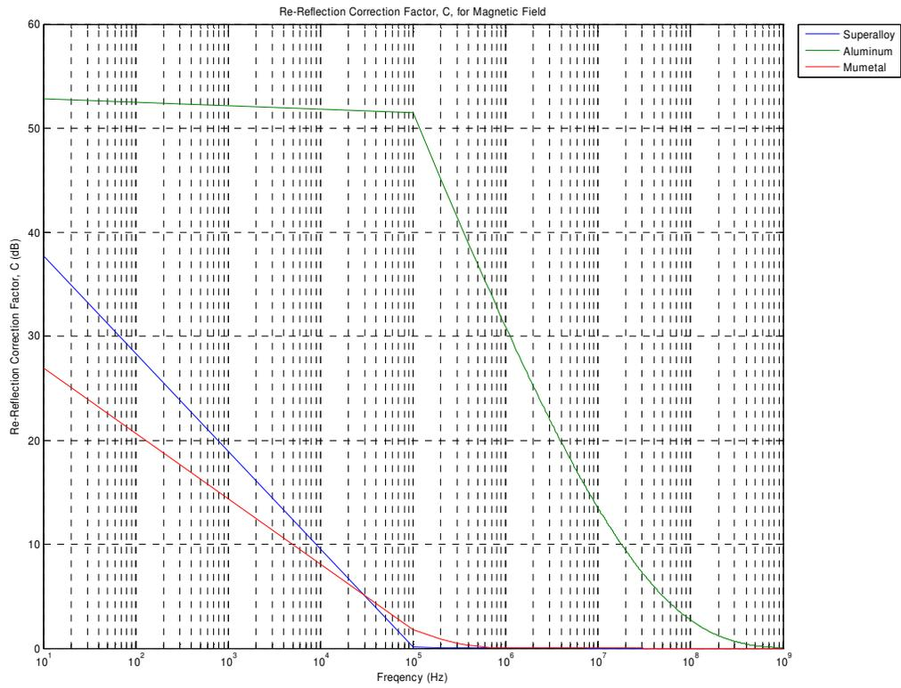
Figure 14. Re-Reflection Correction Factor for Magnetic Field
