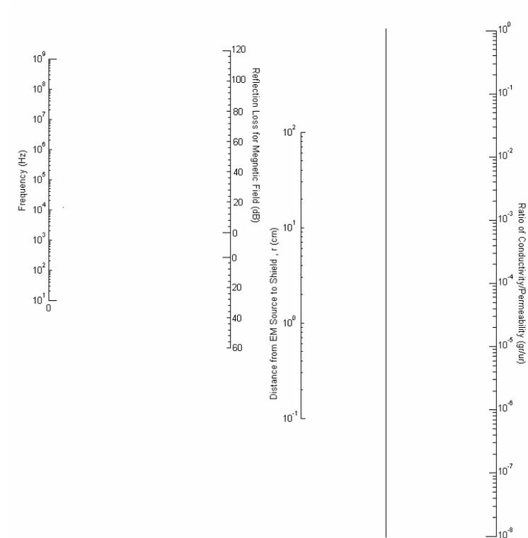
Figure 2a. Reflection Loss Nomograph for Magnetic Field
