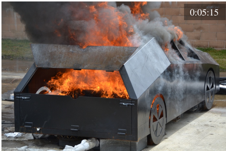
Figure 67 Test A3: ignition (top left); rear involved (top right); fully involved (bottom left); burners off (bottom right)
