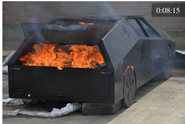
Figure 67 Test A3: ignition (top left); rear involved (top right); fully involved (bottom left); burners off (bottom right)
