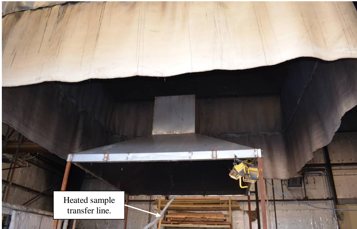
Figure 3. Gas Sampling Hood and Large Calorimetry Hood.
