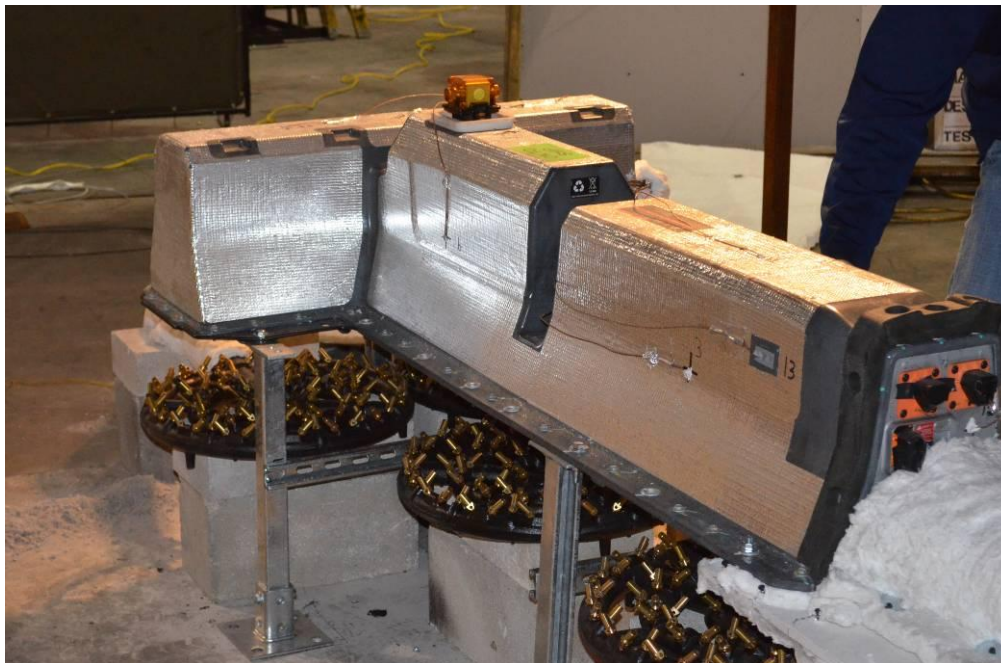
Figure 1. Electric Vehicle Lithium Ion Battery.
