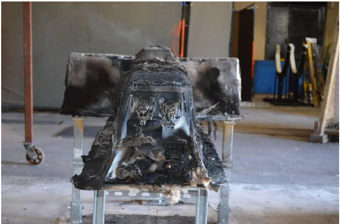
Figure A-14. Post-Test View of Battery.
