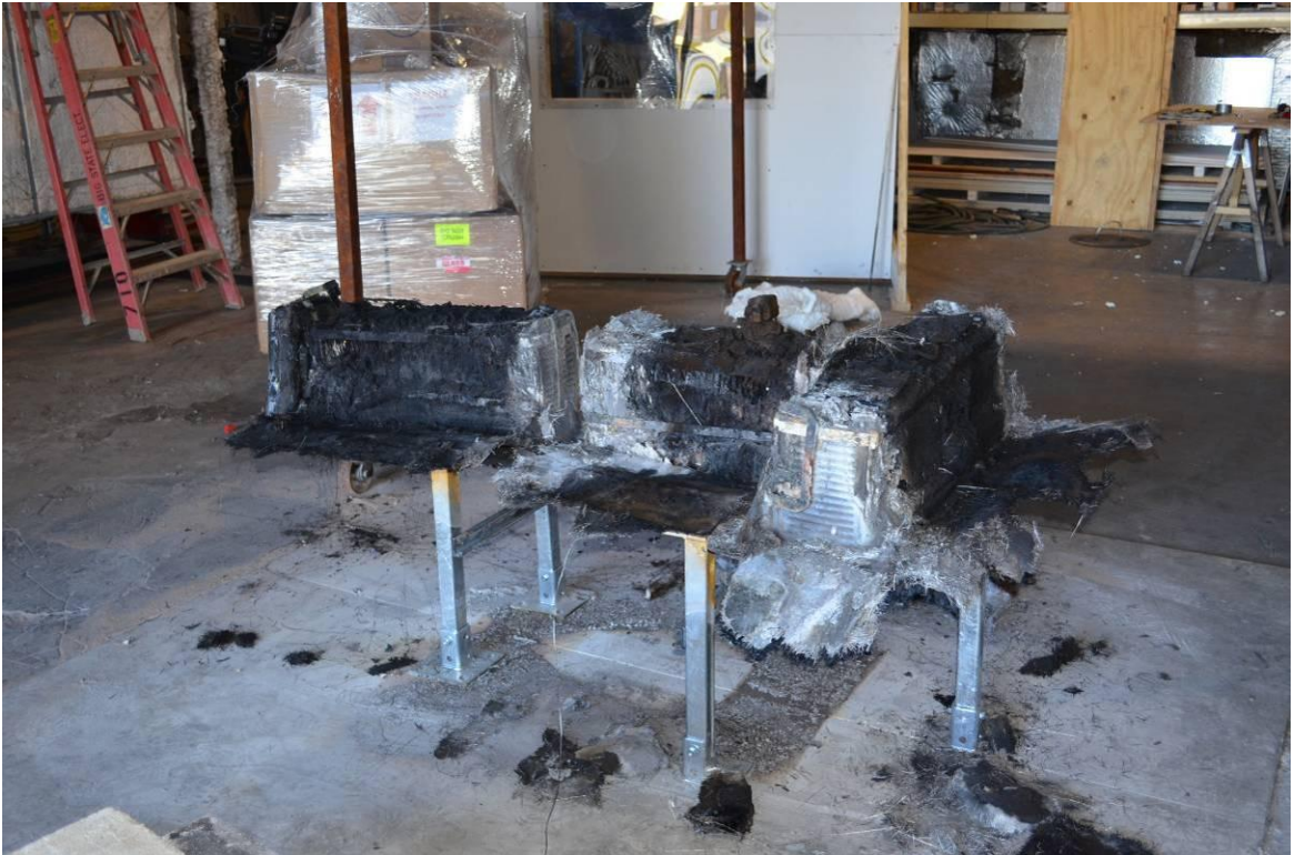
Figure A-15. Post-Test View of Battery (Dissected).
