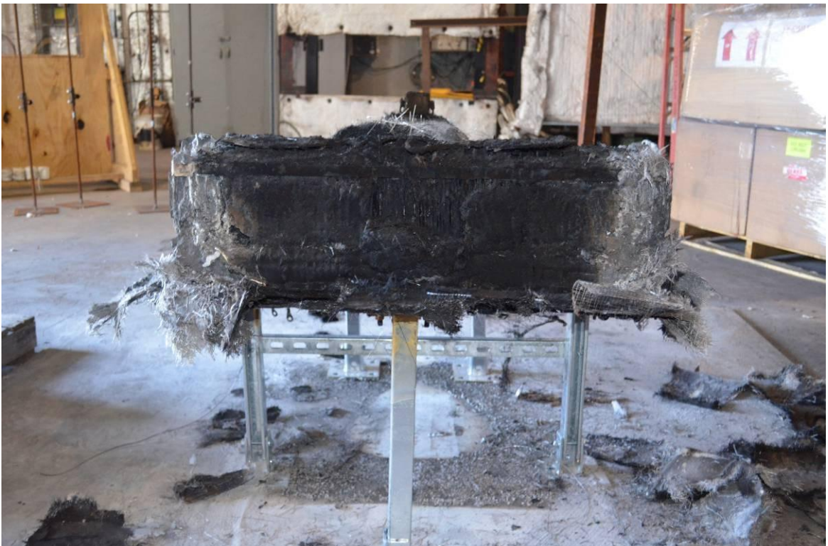
Figure A-16. Post-Test View of Battery (Dissected).
