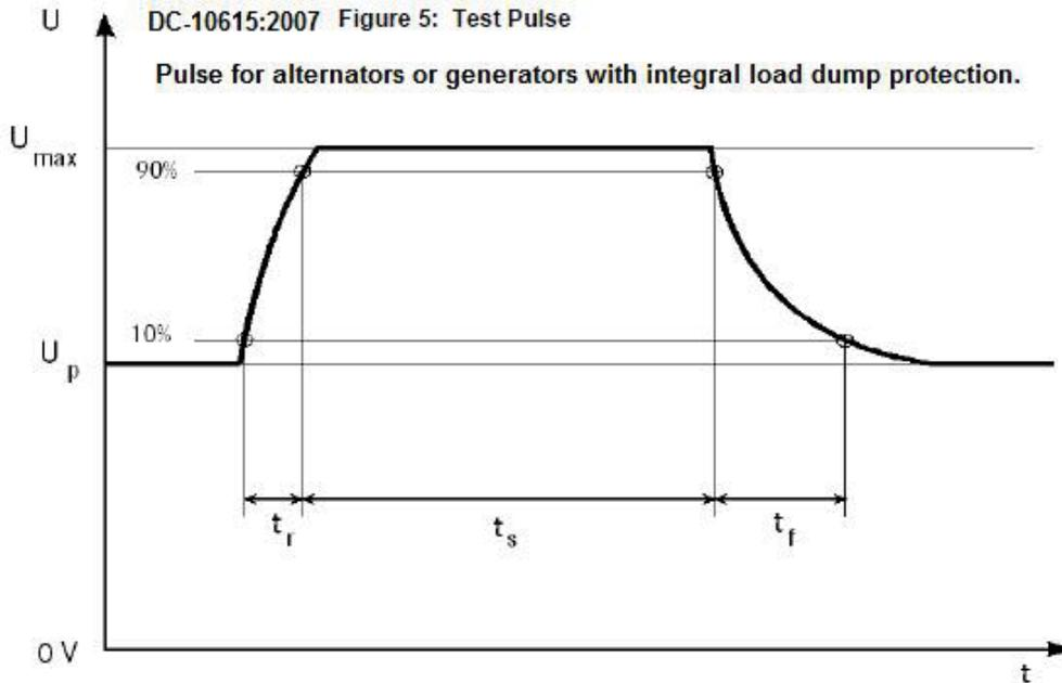
**Table 7: Load Dump Test Pulse Parameters**
