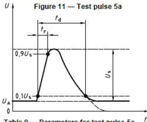
Table 9 — Parameters for test pulse 5a
