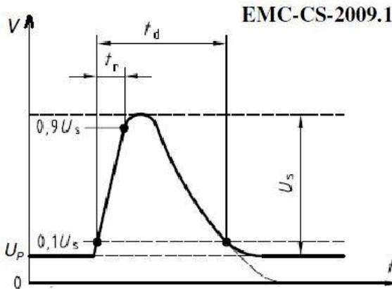
Figure D-10: CI 220 Pulse G2 Characteristics
