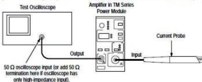
**CAUTION.** Handle current probes with care. Do not drop a probe or subject it to impact, or the core may crack. Do not connect or disconnect a current probe while the probe is clamped around a live conductor, or while the AM 503B and AM 5030 is powered on, or the probe may suffer electrical damage.
