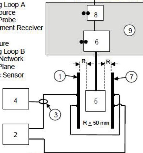
**Configuration for Testing DUT only**
