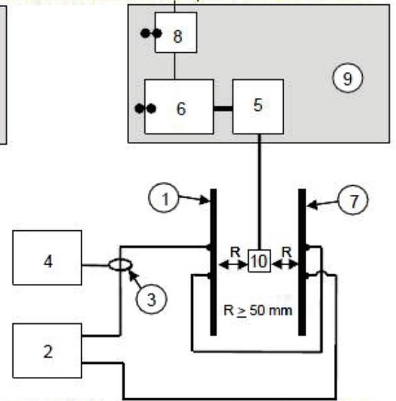
**Configuration for Testing DUT with attached Magnetic Sensors**
