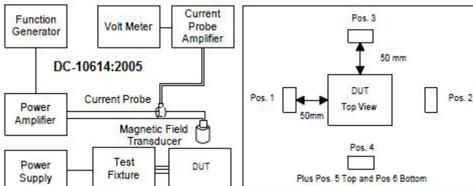
**Figure 19: Magnetic Immunity Test Setup**
