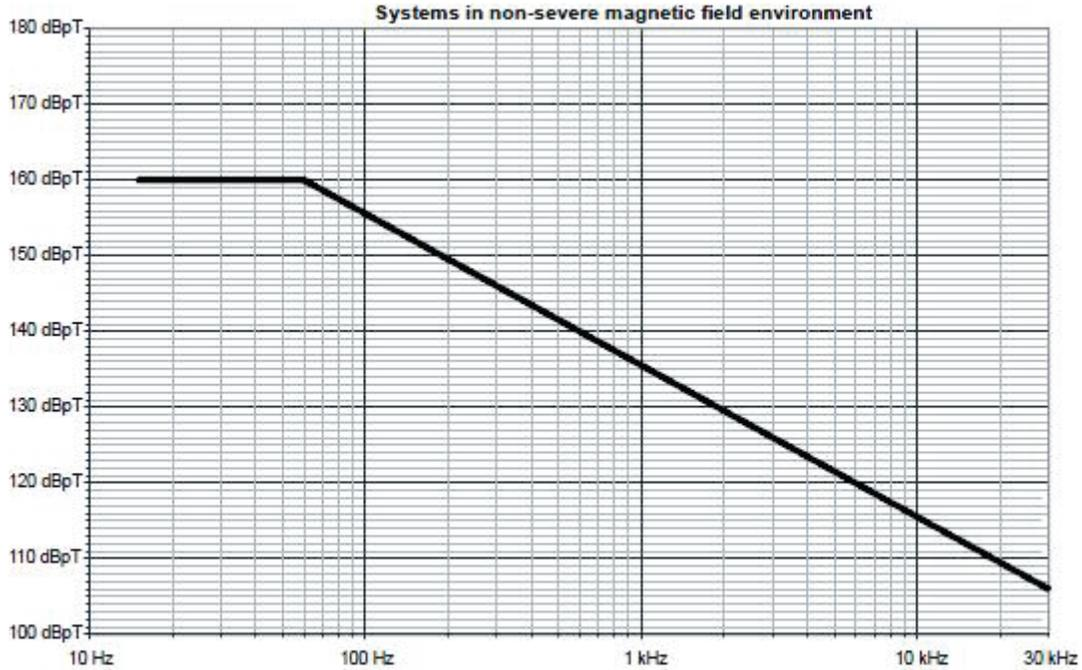
**Figure 16: Test Levels for DUTs in a non-severe magnetic field environment**
