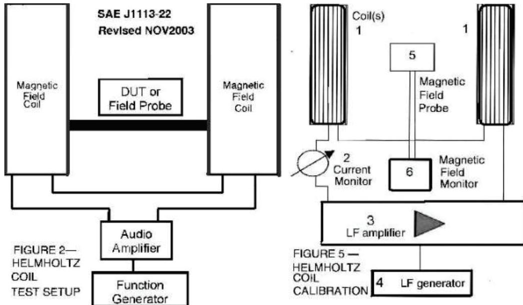
The current carrying capability and number of turns of the coil should be selected such that the test specification can be met. The coil should not have a self resonant frequency at or lower than the upper harmonic frequency of 30 kHz.
