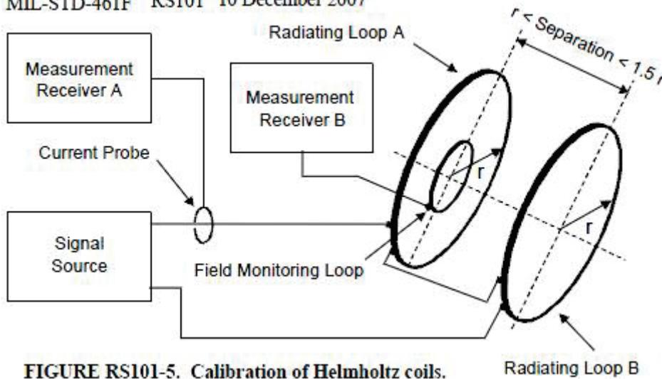
**FIGURE RS101-5. Calibration of Helmholtz coils.**
