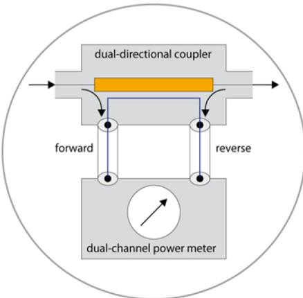
A power amplifier delivers *forward* power into its output cable, which couples this to the load transducer. A mismatch at the load will reflect part of this power back down the cable; this is called *reverse* power. The difference between the two is the *net* power and is passed through the transducer to apply the disturbance to the DUT.
